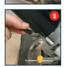
4. Tighten the bevel adjustment lever (8) to secure the base plate.
